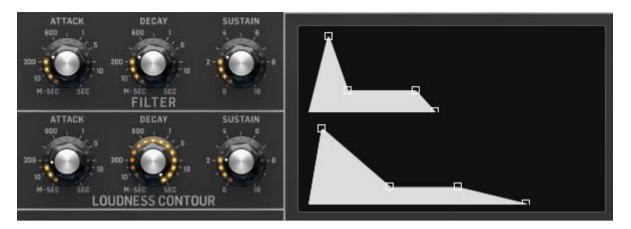
When moving the anchors, the corresponding ADS encoders will also turn and the parameter name and value be displayed in the screen of the top panel area.
